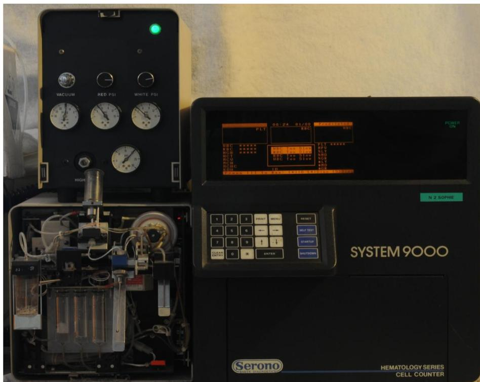
Capacity of measuring a volume range up to 400  $\mu\text{m}^3$
