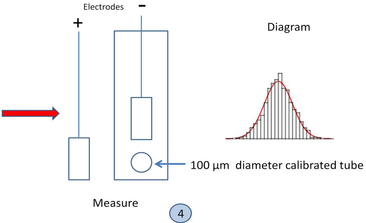
Densitometer allowing the measurement and the adjustment of spores suspensions, in order to standardize the quantity in the sampling probe.
