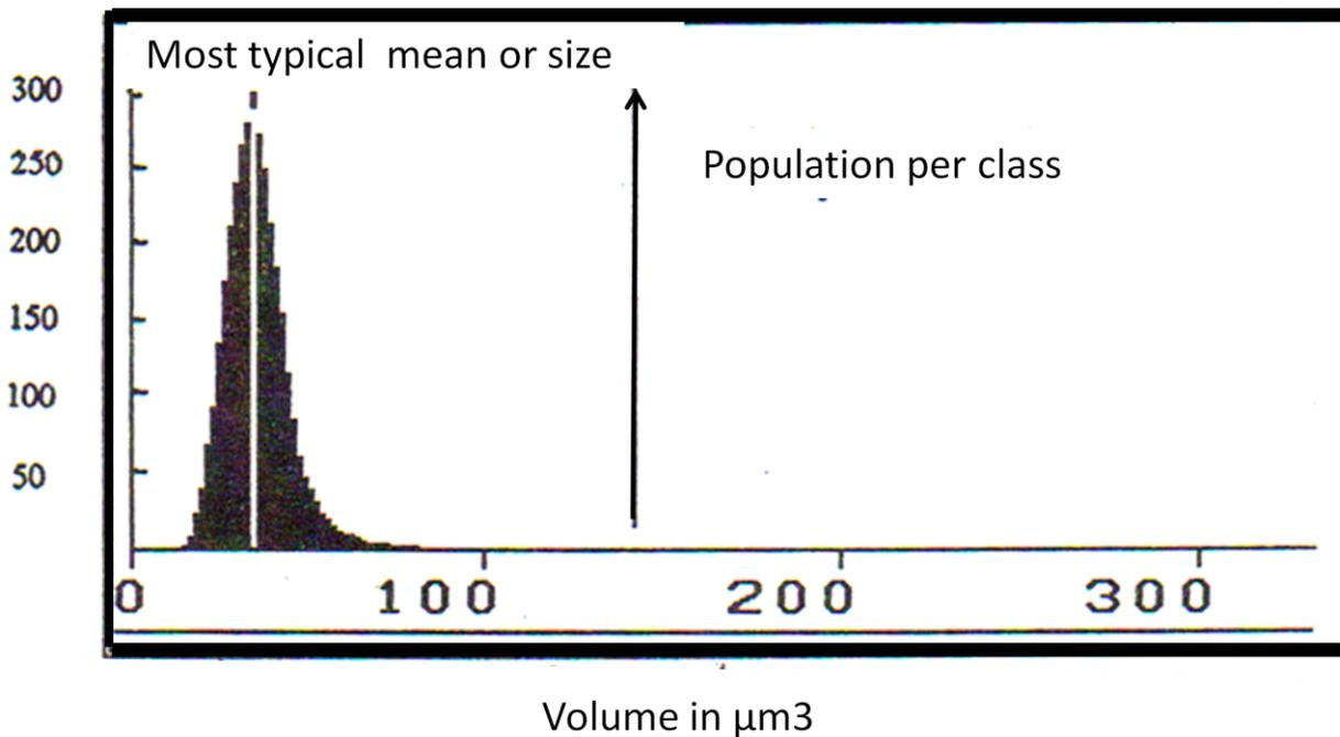
The number of the measured spores varies in the range from 3000 and 10000. This example shows the profile of the spore population. This model of presentation will be used for all measurements.
